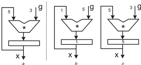
**Fig. 5** Applying a desired test vector to a self-loop
