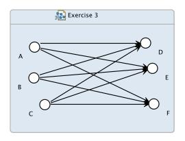
**Exercise 3:** Design a circuit for a protocol among 3 producers and 3 consumers, where a message sent by a producer is synchronously received by all consumers
