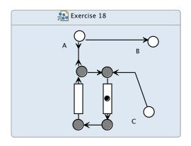
**Exercise 18:** Design a circuit for a protocol among a producer, a consumer, and a regulator, where the producer sends messages to the consumer until the regulator sends a signal
